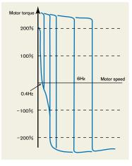
Example torque characteristics of VFA7-2037PL with a 4P-3.7kw stardard motor.
