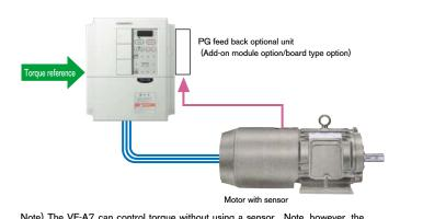
Note) The VF-A7 can control torque without using a sensor. Note, however, the its control accuracy deteriorates under low-load, or low-speed conditions.
